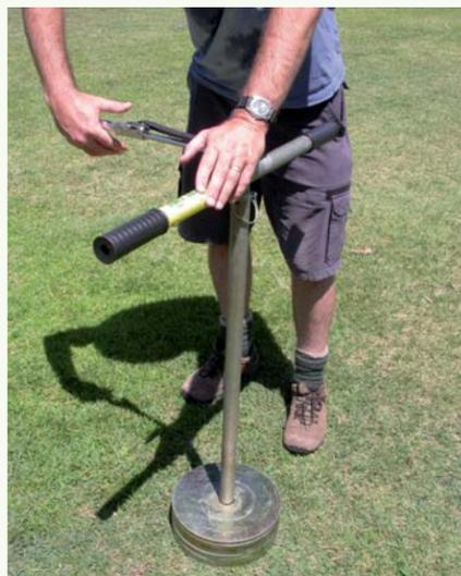
The conventional studded disc apparatus used to measure traction
