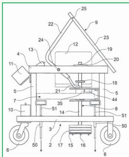
Figure 1. Diagrammatic representation of the QDPI&F automated turf tester
