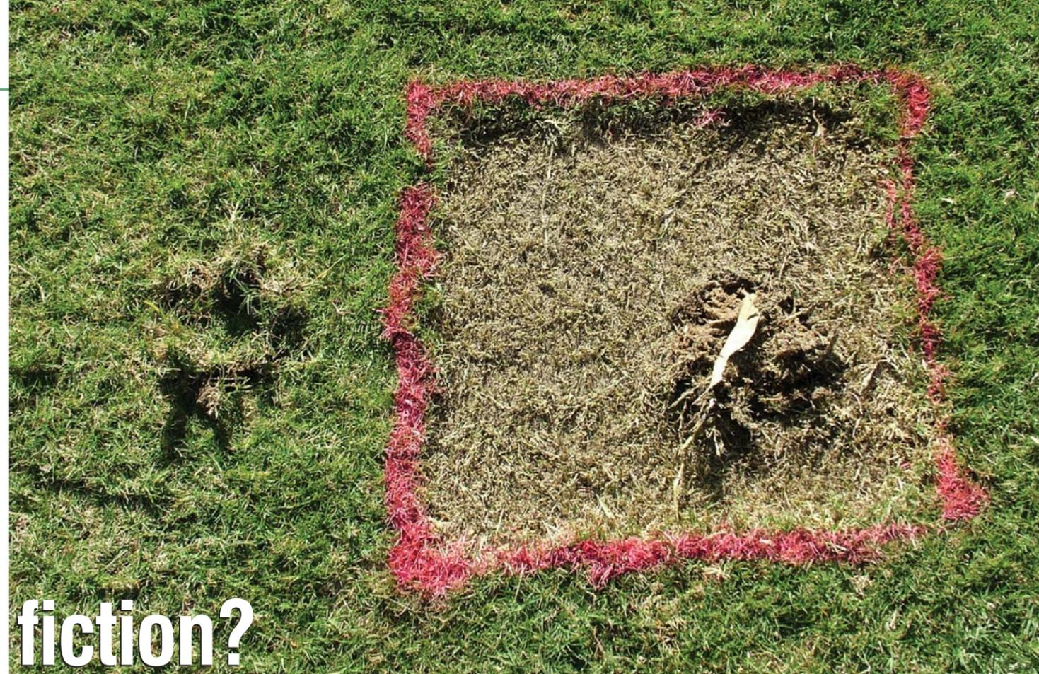
The QDPI&F's Turf Research Group has been undertaking trials, using its specially designed automated traction tester, to determine the influence of thatch on traction. Plots containing a thatch layer (left) and no thatch (within the pink highlighted area) were subjected to traction testing at four to five week intervals during the winter-early spring period in 2006 and 2007
