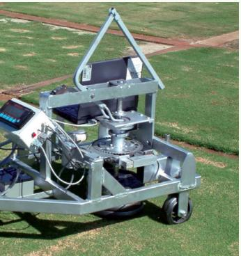
With the exception of kikuyu, all of the way that rotational traction (torque) built up to peak levels. The major difference we found was that some reached peak traction at a lower value and therefore peaked earlier than others which reached higher traction levels (Figure 2). Even weakened couch oversown with ryegrass followed a similar pattern (Figure 3). Traction in
