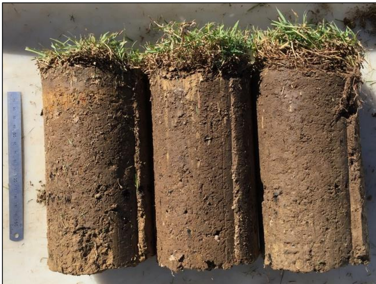
Plate 2 Soil core samples taken from Test Locations 1, 3 and 4 (left to right) to a depth of 200 mm.
