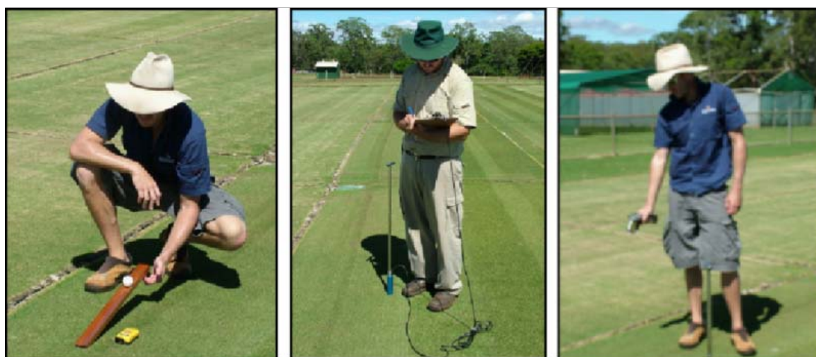
Plate 11. Use of (left to right) a modified stimpmeter (0.64 m long), soil moisture probe and non-contact digital thermometer to measure golf ball roll distance.
